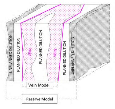
Figure 12-1: Dilution Schematic
